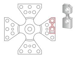
Figure 1 – Hour-glass specimen geometry.
