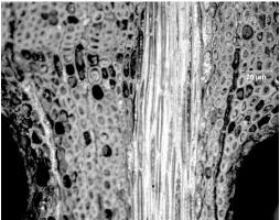
Figure 1 – Showing potential for natural speckle of wood (pine) at x50 magnification using unique timber surface features
