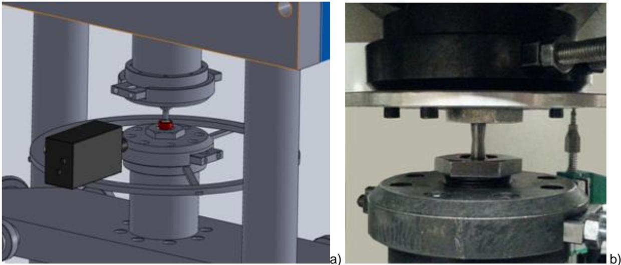
Fig 1: Scheme of the 360-deg measurement system (a) and testing machine used to perform tensile/torsion tests (b).
