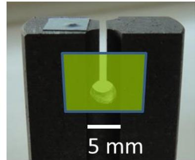
Fig. 1:  $\phi 4$  mm keyhole notched sample for wedge loading. Radiograph FOV highlighted.
