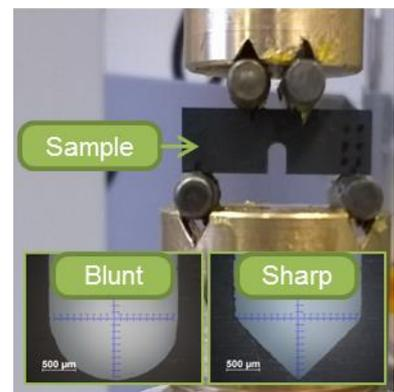
Fig. 2: Short beam flexure sample in loading rig. Sample is 6x6x19 mm. *Inset* Blunt and sharp notch tip micrographs.
