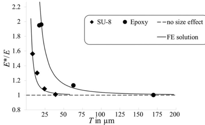
Figure 1: Mean-values of experiments (after Eq. (2)) on epoxy and SU-8, including smoothed FE results.
