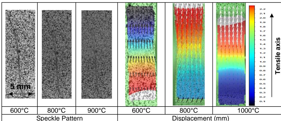
**Figure 1: Comparison of speckle pattern contrast at various temperatures as well as deformation map in the tensile direction**
