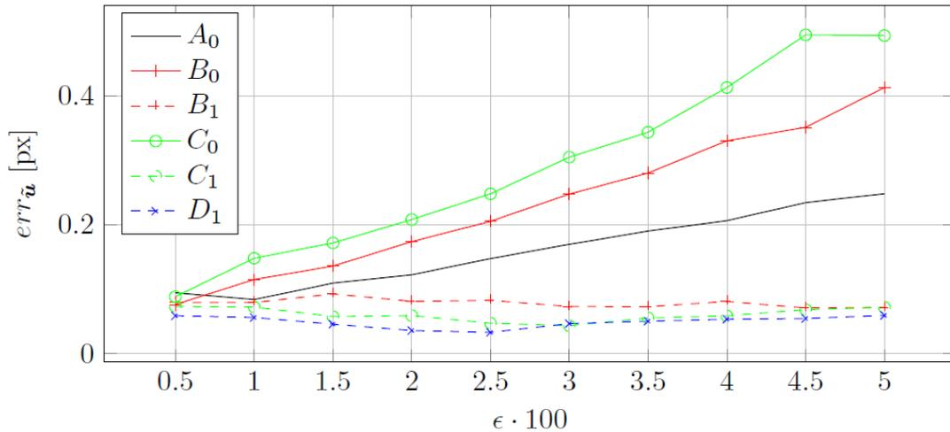
**Figure 3: Maximum error of local subset displacement plotted as function of the applied loading (uniaxial straining) evaluated for different method parameters (subset size and order of kinematic approximation).**
