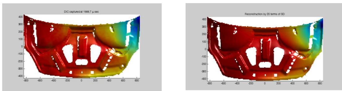
Figure 1. Examples of Measured and Reconstructed Vibration Images
