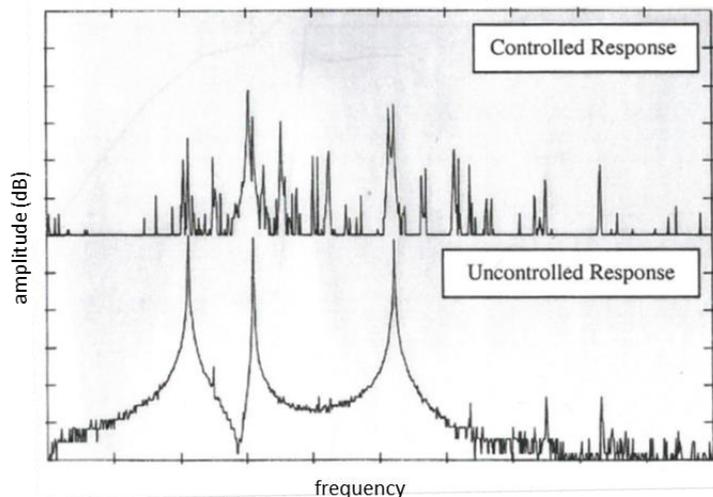
Fig. 4: Effect of active vibration control three modes simultaneously
