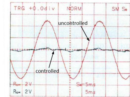
Fig. 2: Effect of active vibration control
