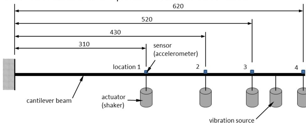
Fig. 1: Test Structure for Active Vibration Control
