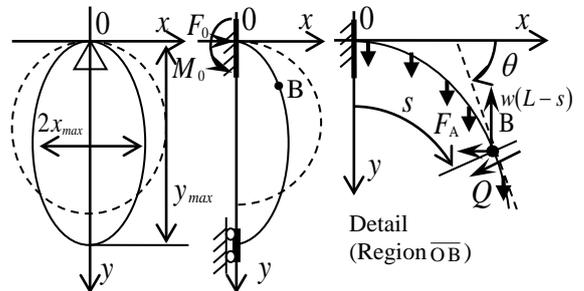
Fig.1 Large deformations of a circular ring subjected to own-weight.
