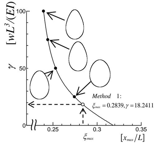
Fig.2 Non-dimensional chart for finding the parameter  $\gamma$  when the deflection  $x_{max}/L$  is given.
