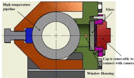
Figure 1. Section of the apparatus for creep strain measurement using inert gas and silver O'ring sealing
