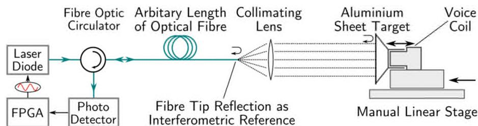
**Figure 1** Illustration of the optical setup and experimental configuration, with a vibrometry test signal induced by a voice coil and with a long-travel movement introduced using the manual linear stage.
