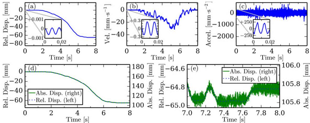
**Figure 2** Measurements using interferometric phase data in (a), (b) and (c), showing relative displacement, velocity and acceleration, respectively. (d) Illustrates the overlap between absolute displacement data, with units indicated on the secondary y-axis, and the relative data of (a), with a zoomed version of this in (e).
