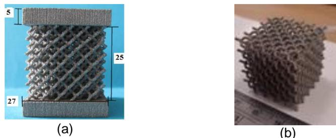
Fig. 1: Designed compression samples with the diamond lattice structure and solid plates (dimensions are in mm)
