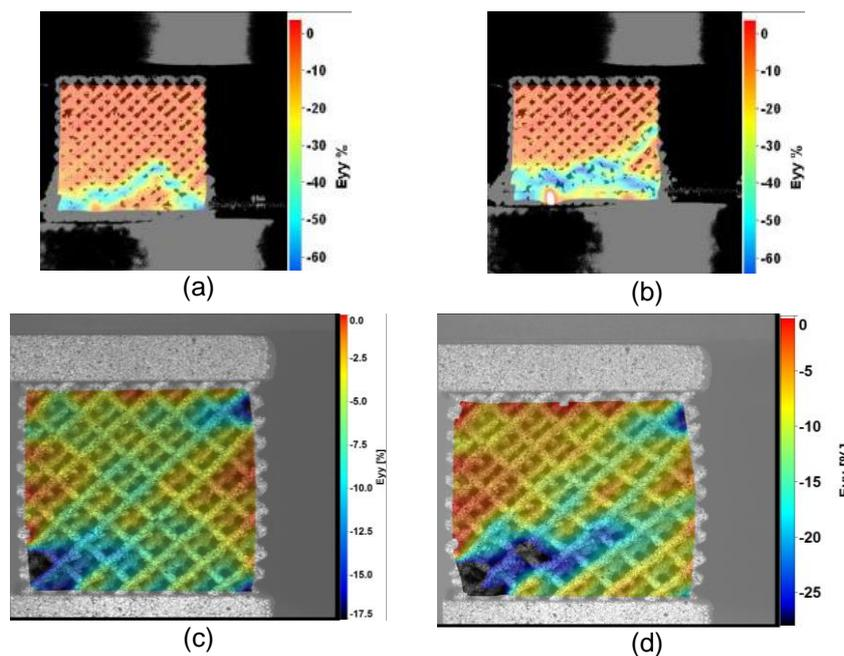
Fig. 2: (a, b) Development of strain localisation within the sample type 1 and (c, d) sample type 2 subjected to compression showing deformation localisation in bands at about  $45^\circ$  with respect to the loading direction (vertical in the figures)
