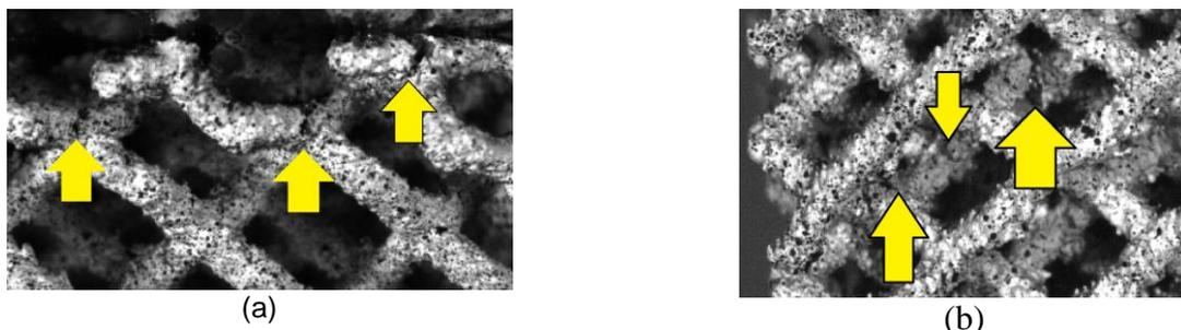
Fig.3: Damage initiation at nodal locations in samples (a) without and (b) with solid plates attached to lattices
