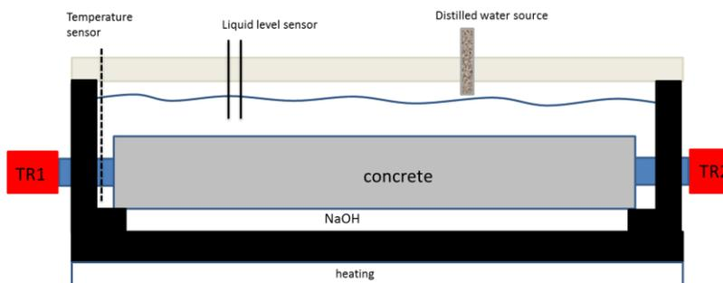
Figure 1: Technical layout of heating chamber equipped with waveguides and ultrasonic sensors.
