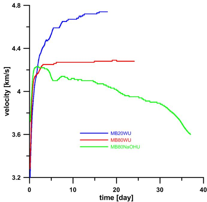
Figure 3: Experimental data of mortar bars obtained by measurements in a temperature-controlled heating chamber – velocity/time dependence.
