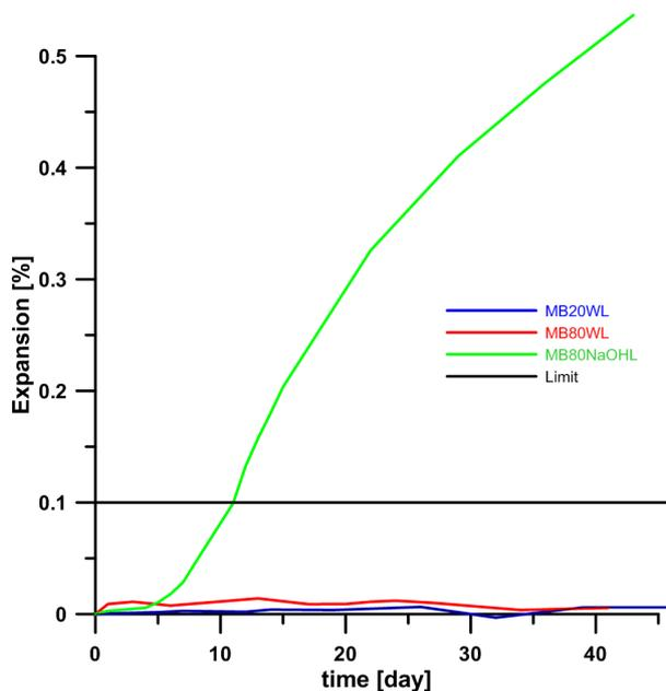
Figure 2: Expansion curves of mortar bars. MB20WL - mortar bars stored in water at 20°C (blue), MB80WL - mortar bars stored in water at 80°C (red), MB80NaOHL - mortar bars stored in 1 M NaOH solution at 80°C (green).
