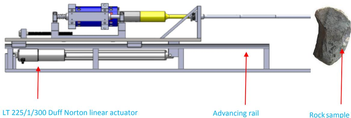
Fig. 3: Experimental test rig for validating the rock coring control strategy.
