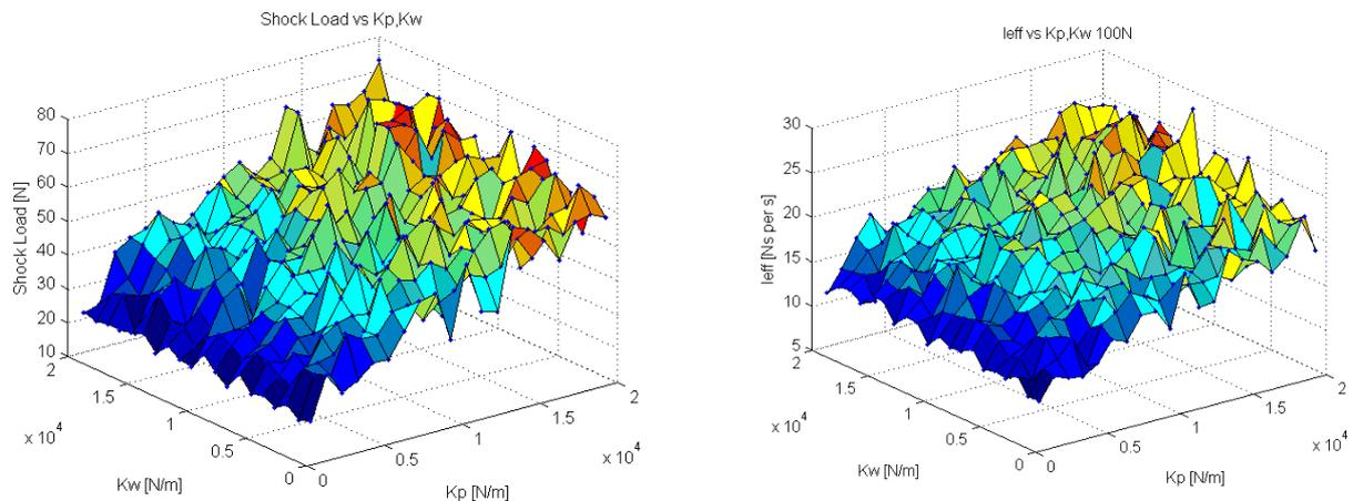
Fig. 1: Predicted transmitted shock load and effective impulse for different back and front spring stiffness.
