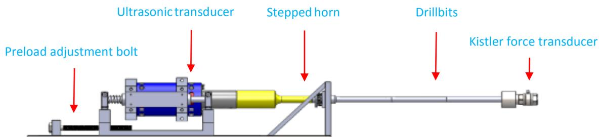
Fig. 2: Experimental test rig for validation of the UPCD dynamic model.
