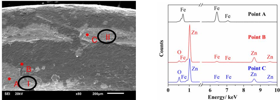
Fig. 2 SEM morphology and EDX patterns corresponding to wear scar of the first thread surface ( $M_0=30 \text{ N}\cdot\text{m}$ ,  $A_F/2=10 \text{ kN}$ ,  $N=10^6$  cycles)
