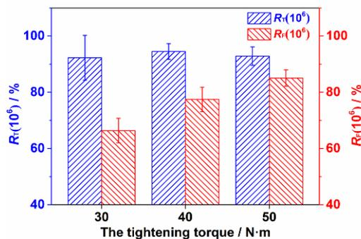
Fig. 4 Self-loosening curves for varying tightening
