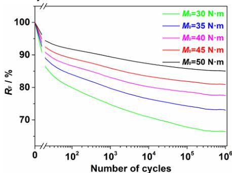
Fig. 3 Self-loosening curves for varying tightening torques
