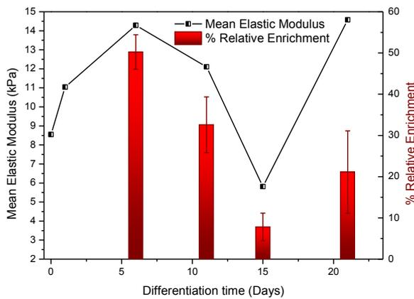
Figure 2 – Variations in mean elastic modulus (Y-axis on the left) of H1-MP cells during osteogenic differentiation (X-axis) are plotted in relation to the percentage depletion obtained in the permeate for an H1-hESC/osteocyte mixed cell population run once through our elastic-modulus based separation device, at the indicated days during differentiation.
