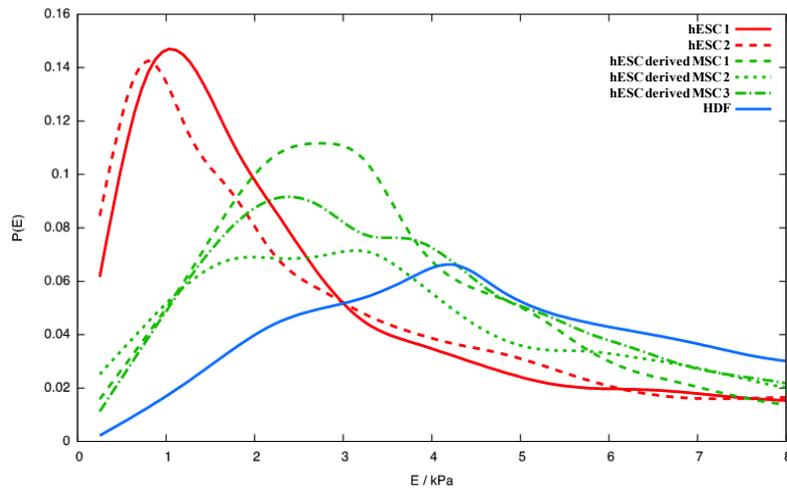
Figure 1 – Variation in elastic modulus as a probability distribution. Red data refers to two different pluripotent cell types, green to three different partially differentiated multipotent cell types (germ layer specified) and blue to terminally differentiated cells. All plots from analysis of >800 force response curves. Data clearly indicates increasing elastic modulus and therefore cell stiffness with cell differentiation, therefore with cell specificity.
