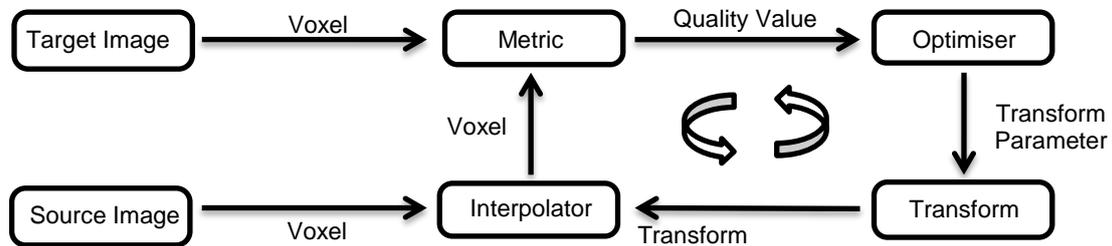
Fig. 1: Graphical representation of the image registration process.
