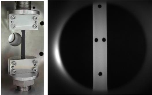
Figure 3: Flat dumbbell polymer specimen and strain measurement by patterning
