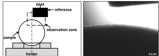
Figure 6: Measurement of dilatation of a spherical specimen in an elastomer under hydrogen pressure
