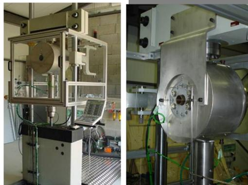
Figure 2: Front and back of the HYCOMAT test rig for mechanical testing under pressurized gas (H2, CO2 and N2)
