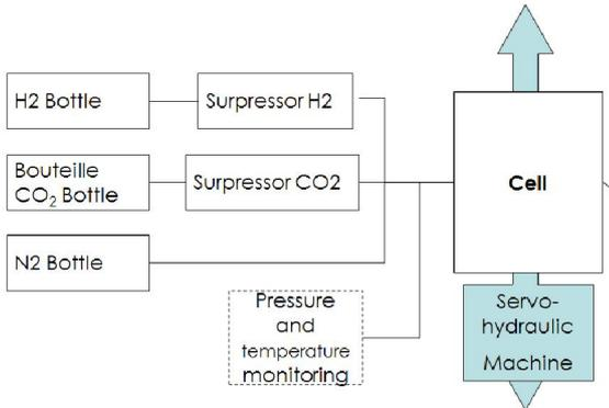
Figure 1: Schematic overview of test rig under pressurized hydrogen, carbon dioxide, nitrogen
