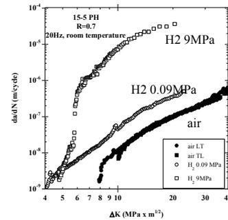
Figure 4:  $da/dN$  vs  $\Delta K$  curves obtained under two hydrogen pressures 0.09 and 9 MPa, compared to the one obtained in ambient air.
