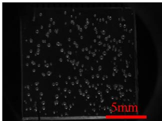
Figure 5: Example of cavitation in an elastomer during decompression of hydrogen pressure
