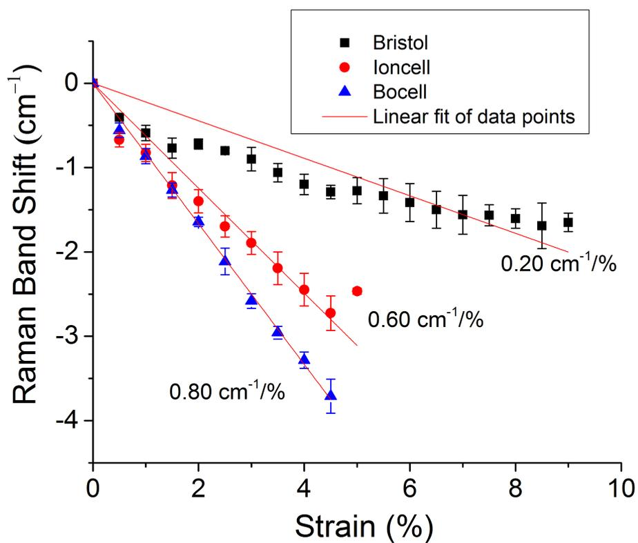
Fig. 1. Shift in the position of a Raman band ( $1095\text{ cm}^{-1}$ ) as a function of deformation for three cellulose fibres
