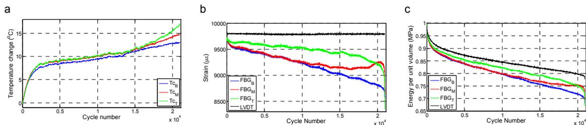
**Figure 1:** Evolution of temperature (a), strain (b) and mechanical energy (c) for all thermocouples and FBG sensors where the subscripts B, M, and T denote bottom, middle, and top locations along the gage length of the specimen.
