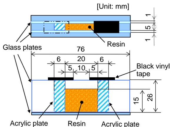
Fig. 1 Shape and dimensions of specimen
