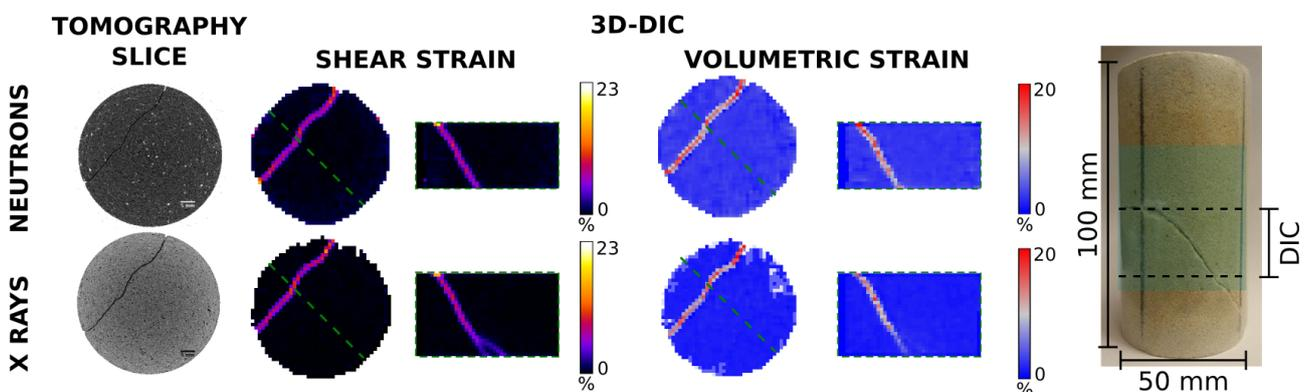
**Figure 1** Reconstructed horizontal slices after deformation from the neutron and x-ray tomographies, the results of the 3D-DIC analysis in terms of maximum shear strain and volumetric strain, and a picture of the sample after deformation.
