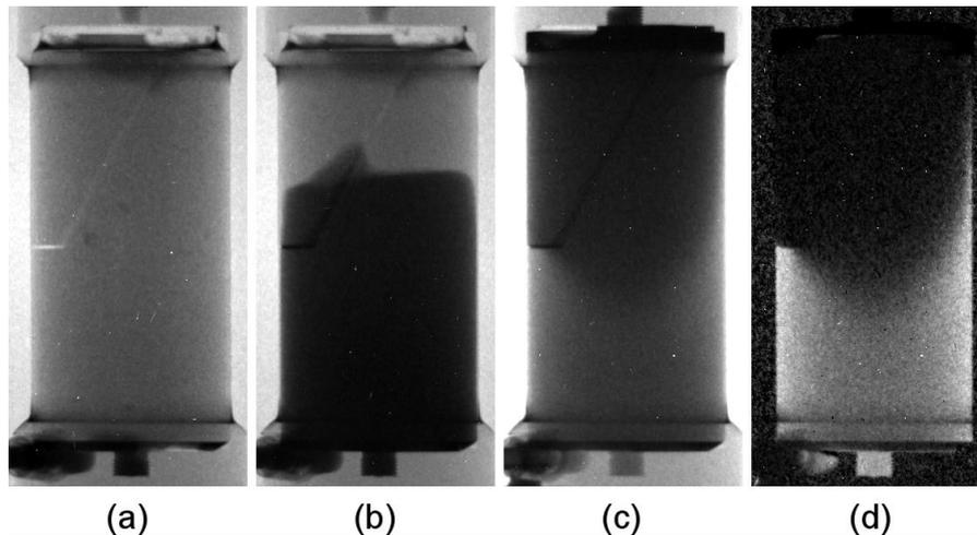
**Figure 2** Neutron radiographies of: (a) a dry sample; (b) an H<sub>2</sub>O/air flow stage; (c) a D<sub>2</sub>O/H<sub>2</sub>O flow stage (H<sub>2</sub>O is dark, i.e., high attenuation) and (d) difference between (c) and a radiography taken before D<sub>2</sub>O entrance to enhance the contrast between fluid phases (black indicates zero saturation change and white replacement of H<sub>2</sub>O by D<sub>2</sub>O).
