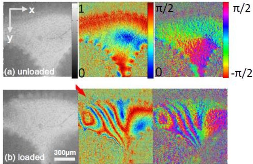
Fig. 1 PS-FF-OCT imaging: *en-face* reflectivity (left), retardation (middle) and axis orientation (right) excerpts, exemplified for a polymer test sample, subjected alternately to a (a) load and (b) unloaded state.
