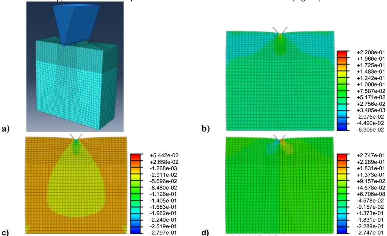
Figure 1: a) Finite element model of the rubber block subject to a 2mm indentation by a rigid wedge and the corresponding strain maps in b) XX, c) YY and d) XY directions.
