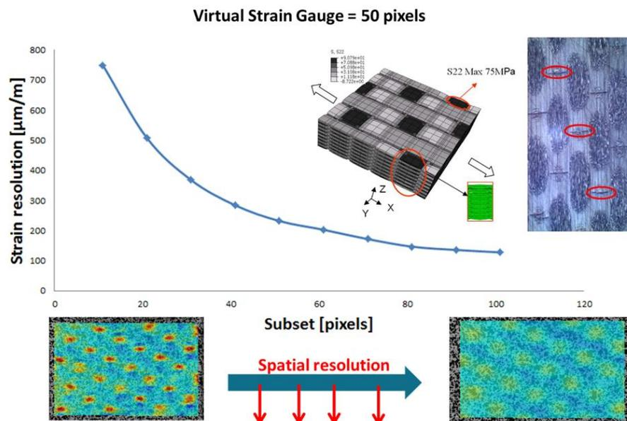
Fig. 1: Impact of subset size on strain noise floor and spatial resolution.
