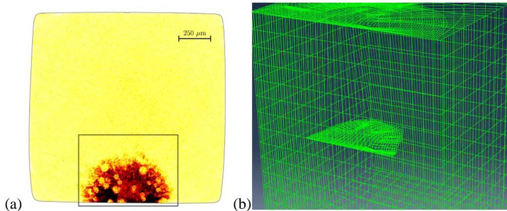
Figure 1. (a) Projection of the correlation residuals [2] (b) Definition of a complex 3D crack geometry for J-integral calculation
