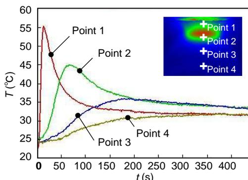
Fig. 4 Time variations of temperature,  $T$ , at points 1 to 4 shown in Fig. 3
