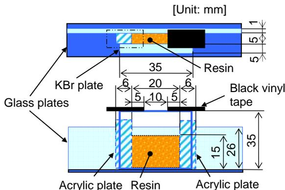
Fig. 1 Shape and dimensions of specimen
