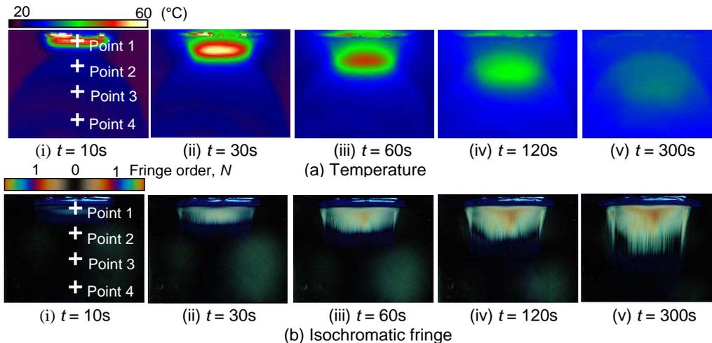
Fig. 3 Time variations of temperature and isochromatic fringe
