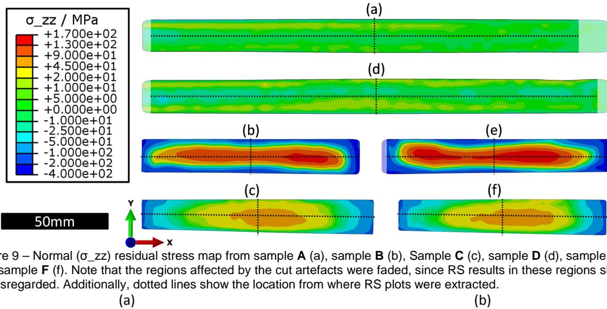
Figure 9 – Normal ( $\sigma_{zz}$ ) residual stress map from sample **A** (a), sample **B** (b), Sample **C** (c), sample **D** (d), sample **E** (e) and sample **F** (f). Note that the regions affected by the cut artefacts were faded, since RS results in these regions should be disregarded. Additionally, dotted lines show the location from where RS plots were extracted.
