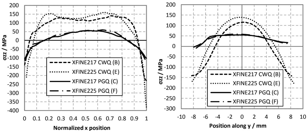
Figure 1 – (a) Normal ( $\sigma_{zz}$ ) residual stress profiles along the normalized x axis at mid-thickness of CWQ and PGQ T6 samples and (b) through the thickness in the centre of CWQ and PGQ T6 samples.
