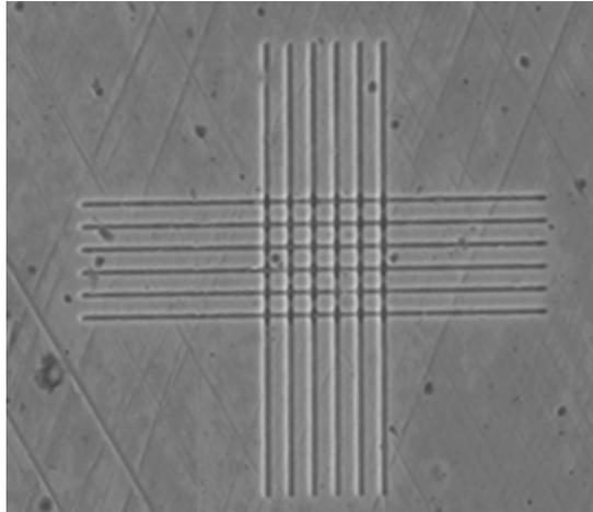
Fig. 2. 6x6 gridline created using Focused Ion Beam on BMG in surface-decoration process
