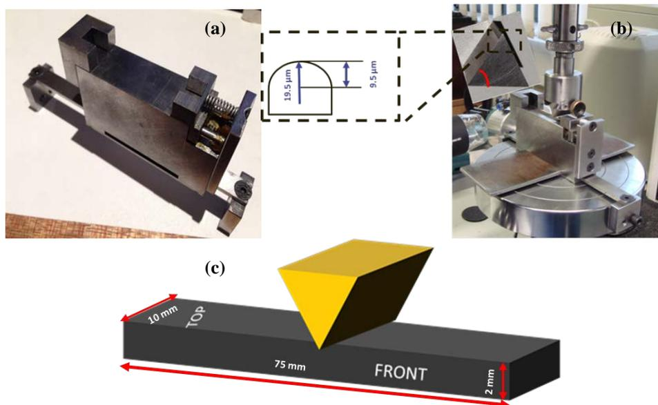
Fig. 1 (a) Designed fixture; (b) experimental setup for wedge indentation (Inset image: wedge indenter and its dimensions) (c) Schematic of wedge-indentation experiment [3]
