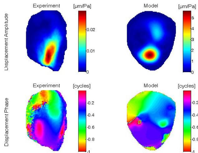
Figure 2: The displacement amplitude (top) and phase (bottom) of the eardrum at 1600 Hz, compared for the holography results (left) and the optimized model (right) [4]. The optimized Young's moduli  $E$  were found to be  $[E_{\text{TM}}, E_{\text{EC}}] = [40.3, 39.6]$  MPa. (TM = tympanic membrane, EC = extracolumella).
