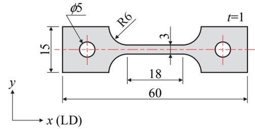
Fig. 1 Shape and size of plate specimen.
