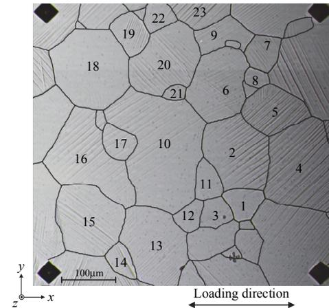
Fig. 2 Measurement area on the specimen surface after tensile test.
