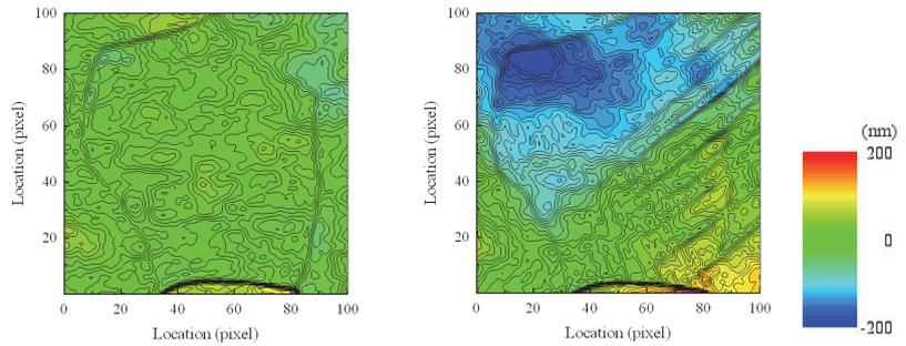
Fig. 3 Height distribution in grain 2 at  $P=0$  (initial) and 635 [N].
