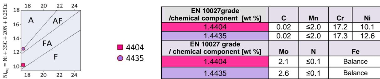
Figure 1 : Solidification mode diagram based on the WRC-1992 diagram [8] (left) and EN 10027 grades 1.4404 and 1.4435 austenitic stainless steel compositions [6].
