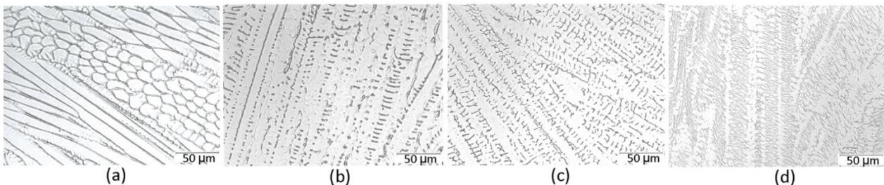
Figure 2: Fusion zone microstructure resulting from solidification mode A (a), AF (b) and FA, skeletal ferrite morphology (c) and lathy ferrite morphology (d) [7]
