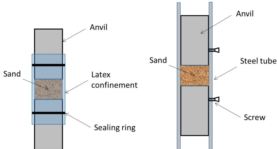
**Fig. 1: Latex (left) and rigid (right) confinement**
