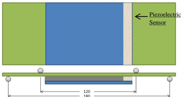
Figure 1: Single Piezoelectric Sensor embedded into the lap joint – Experimental configuration
