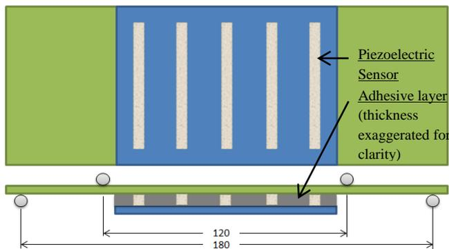
Figure 3: Top view of the piezoelectric sensors within the lap joint - Section of the experimental setup
