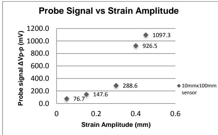
Figure 2: The output probe signal as a function of strain amplitude range
