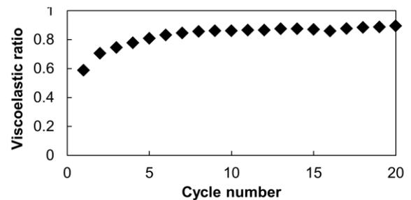
Figure 2: Typical trend of viscoelastic ratio obtained from the indentation test.
