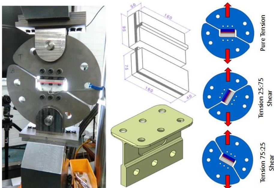
**Figure 1.** Experimental setup demonstrating the Arcan test fixture, initial weldment pieces, final test specimen geometry and the three test configurations for variable loading.
