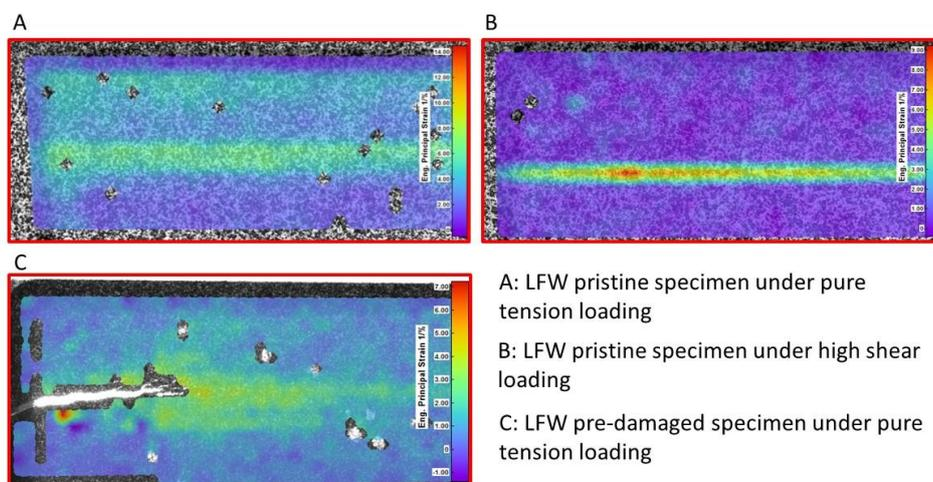
**Figure 2:** Principle strain in the central shear tie pocket, captured immediately prior to failure using Digital Image Correlation, for pristine and pre-damaged specimens under different loading.
