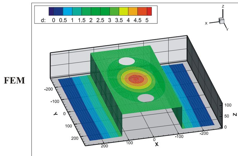
Figure 3: Comparison of 3D displacement fields computed by the present technique (SMS), a 3D DIC technique and a finite element method.
