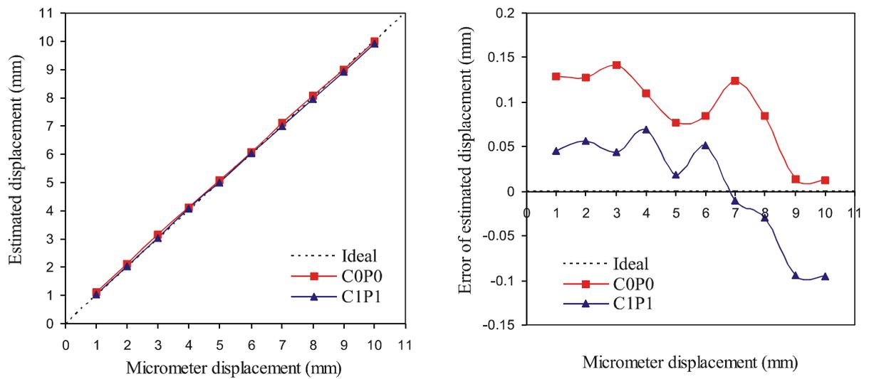
Figure 2: Comparison of estimated displacement at loaded point and micrometer displacement.
