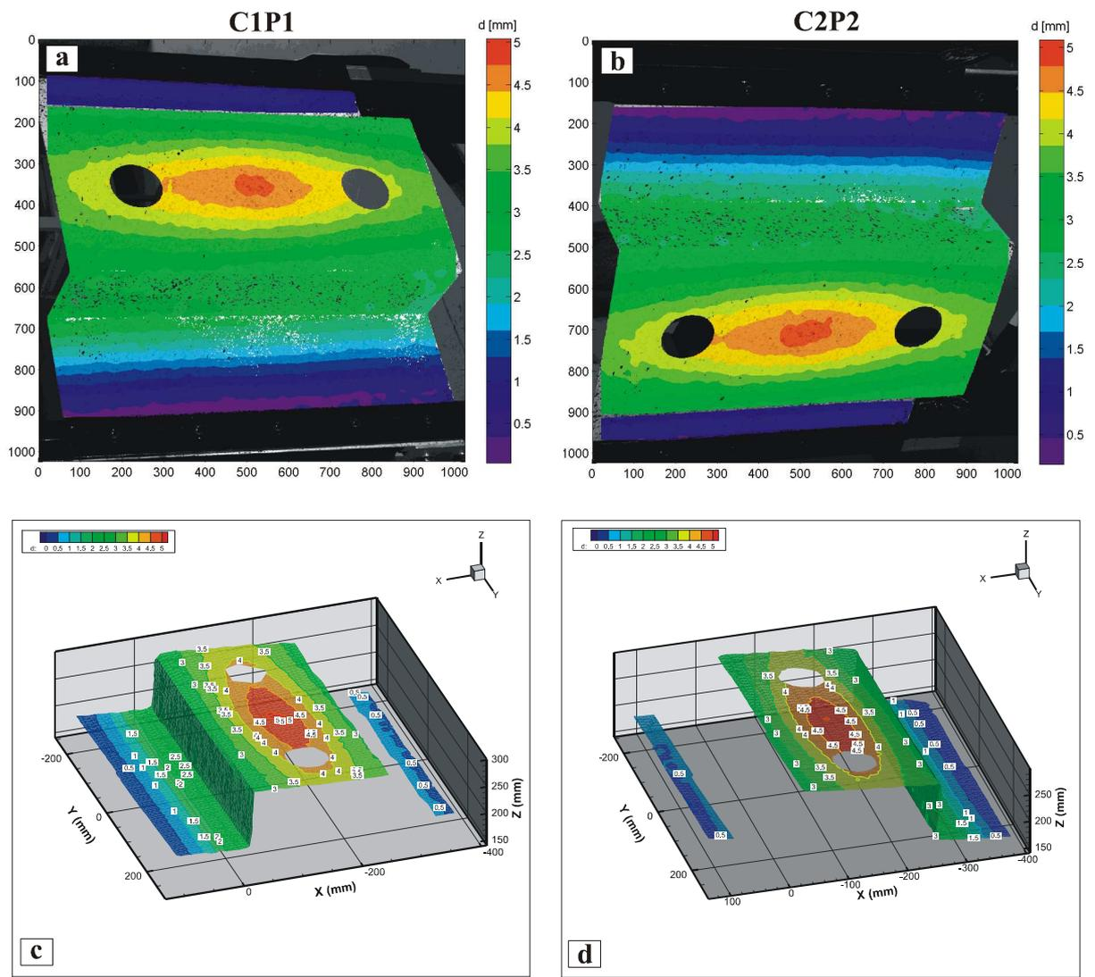
Figure 1: Displacement magnitude fields measured by pairs C1P1 and C2P2, represented on 2D texture images and measured 3D shapes.
