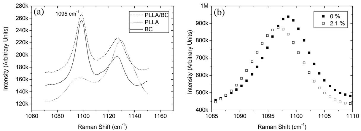
Figure 3: (a) BC/PLLA composite, PLLA and BC in the region close to the  $1095\text{ cm}^{-1}$  band. (b) Shift in  $1095\text{ cm}^{-1}$  Raman band at 0 % and 2.1 % strain for BC.
