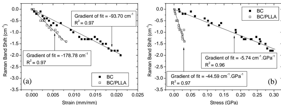
Figure 4: Shifts in the peak position of the  $1095\text{ cm}^{-1}$  Raman band with respect to strain (a) and stress (b).
