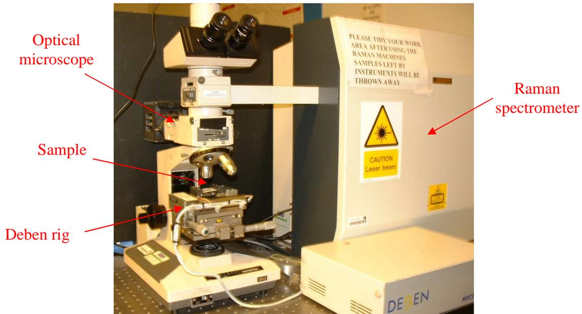
Figure 2: An image showing the experimental set-up in order to perform stress-transfer measurements using Raman spectroscopy.
