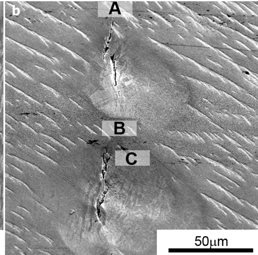
0.9 failure strain. Micro cracks in ASB
