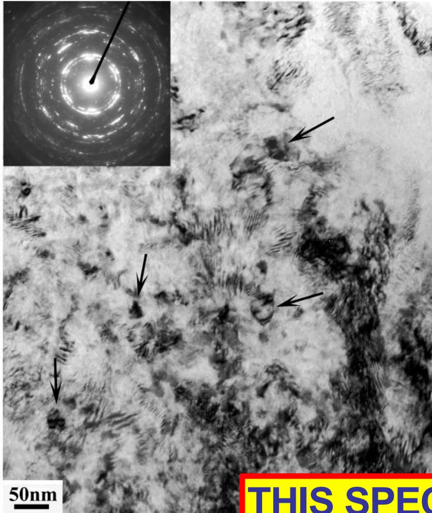
**Dynamically recrystallized grains** (10-30 nm) formed in the highly dislocated area are indicated by arrows.
