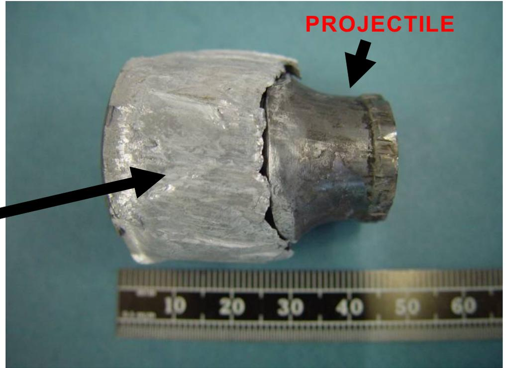
**Plugging failure on the backside of an aluminum alloy armor plate
