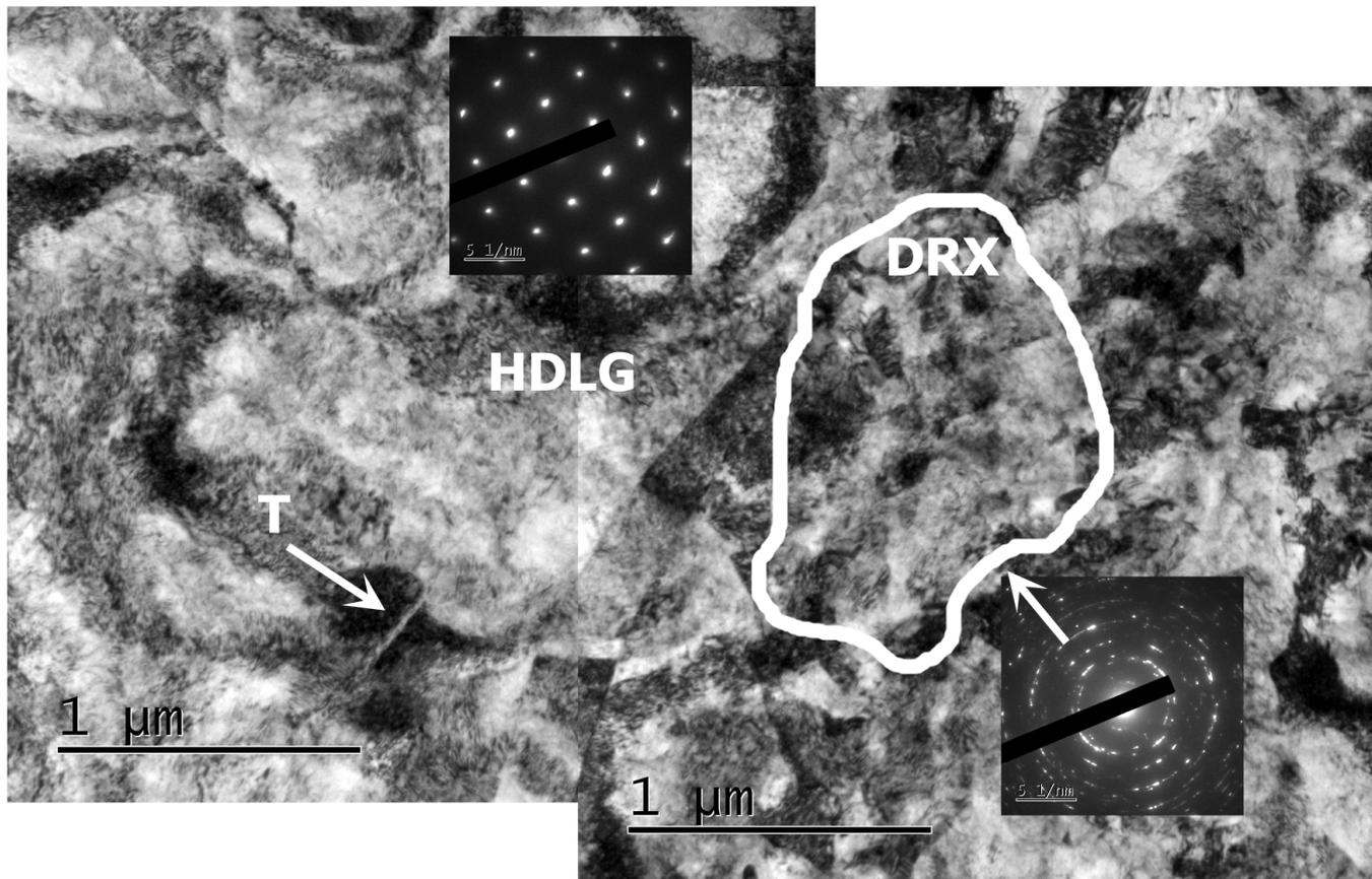
(Box C), ~5 micron aside from the crack. Heavily deformed microstructure with a DRX island within it (marked by the white line), similar to the microstructure observed between the cracks (Box B). A twin is arrowed in the heavily deformed region.
