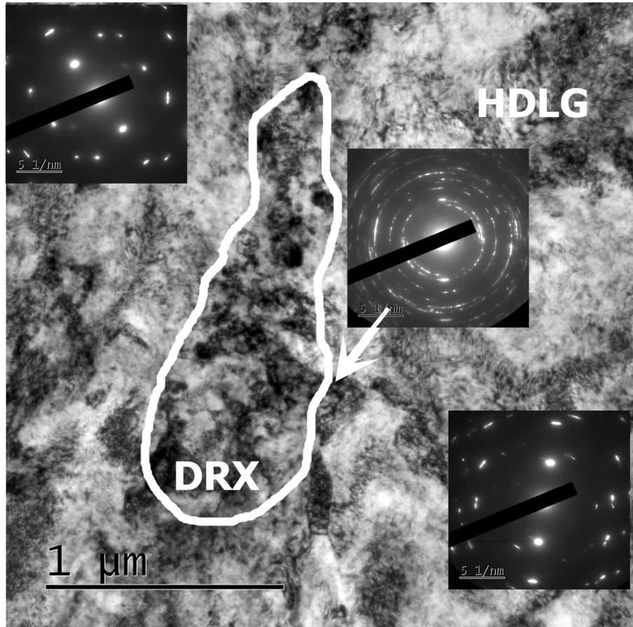
Sample between the cracks (box B): heavily deformed Ti matrix and small DRX'ed regions and highly deformed large grains (HDLG).
