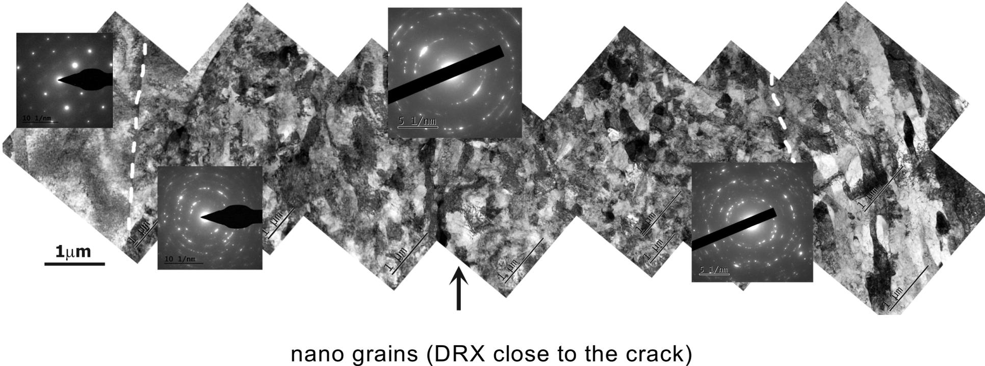
nano grains (DRX close to the crack)
