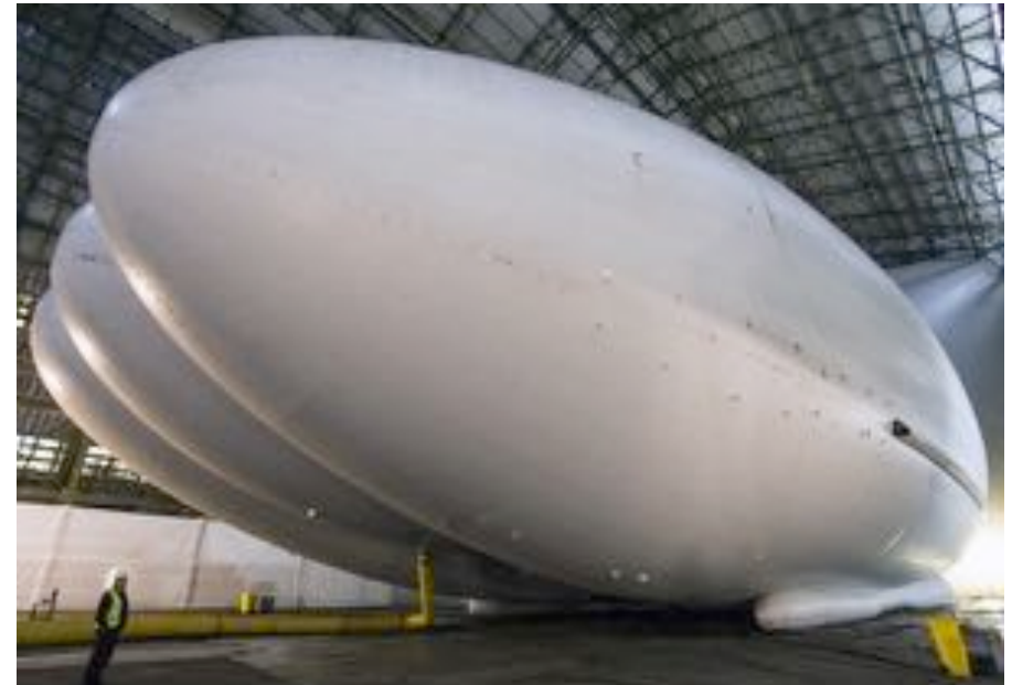
AirLander 50: the lighter than air hybrid airship, originally designed for the United States Army as Long Endurance Multi-intelligence Vehicle (LEMV)
