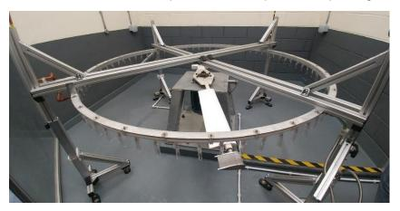
Figure 1- Setup of ETC's Erosion Test Rig
