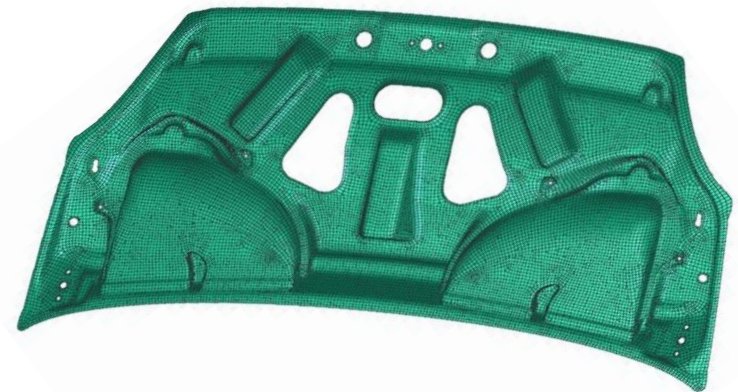
Finite element model of bonnet liner
