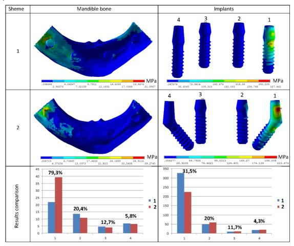
Fig. 2: The von Mises stresses in the lower jaw and implants when chewing. On histograms - the maximum stress values: blue bars – scheme 1, brown – scheme 2; the percentage indicates the difference between the schemes.
