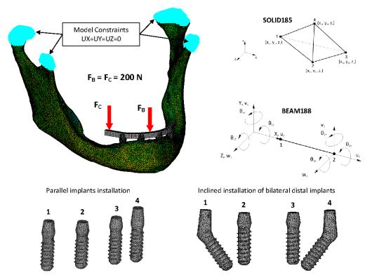
Fig. 1: Mandible finite element model in the biting and chewing processes modeling and model constraint conditions (top left); finite elements types used to create the model (top right); implants placement schemes (below)
