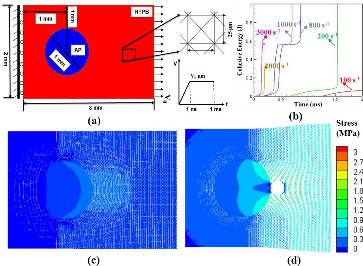
Figure 2. (a) Schematic of Finite Element model (b) Cohesive energy of the system failure with time for different strain rates and Stress distribution at 87.5 μs for (c) 1000 s<sup>-1</sup> and (d) 10000 s<sup>-1</sup>.
