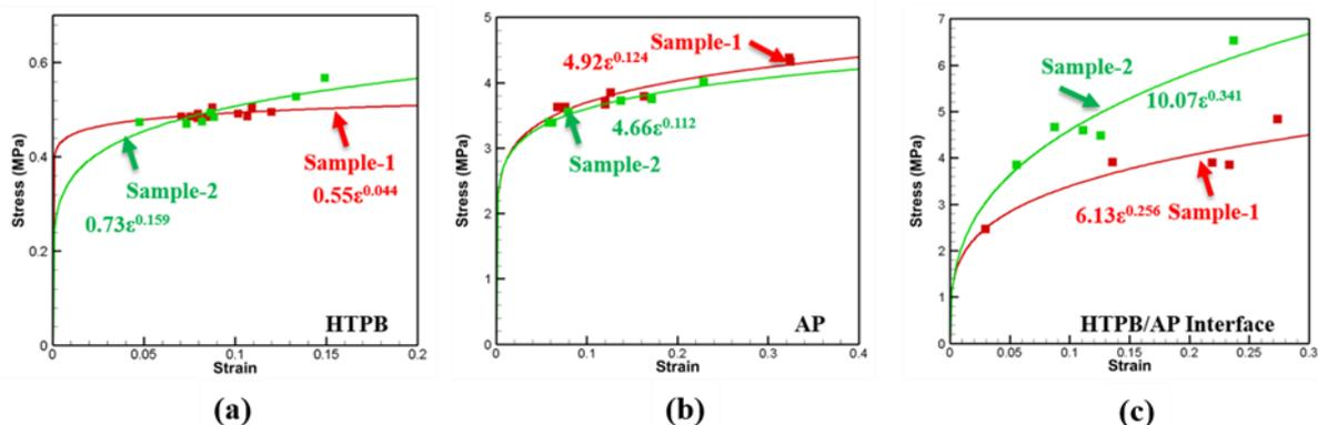
Figure 1. Stress-strain response of (a) HTPB, (b) AP and (c) Interface for sample without binding agent (Sample-1) and with binding agent (Sample-2).
