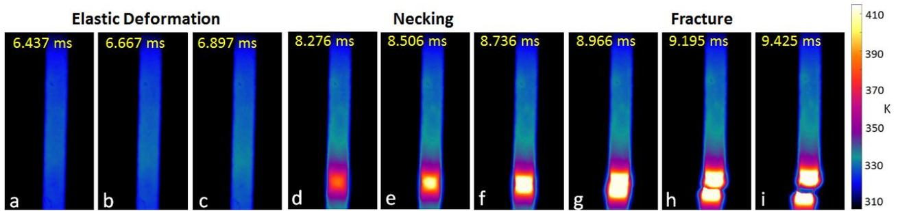
**Figure 1.** Selected infrared images recorded during a tensile stress test carried out on a steel sample.
