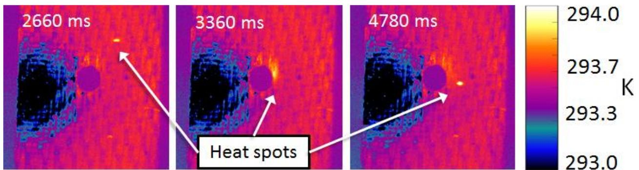
**Figure 2.** Selected frames recorded during a tensile test carried out on a carbon fiber composite material highlighting the presence of cracks within the epoxy-polymer matrix.
