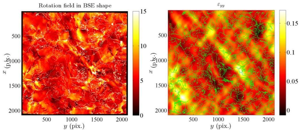
Figure 3. Crystal rotation (left) and strain along the tensile direction (right) between initial and final states. Grain boundaries are shown as green lines in (right). Significant and similar concentration is visible in both images.
