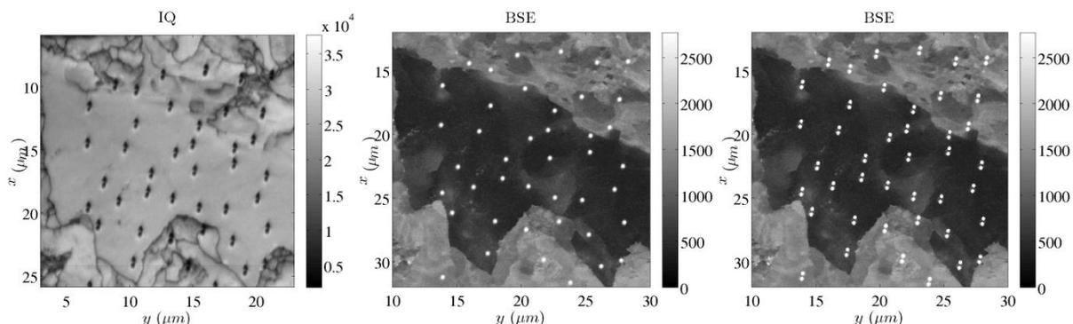
**Figure 1.** Speckle shown in IQ images (left) after tilt correction, raw BSE (middle) and transformed BSE
