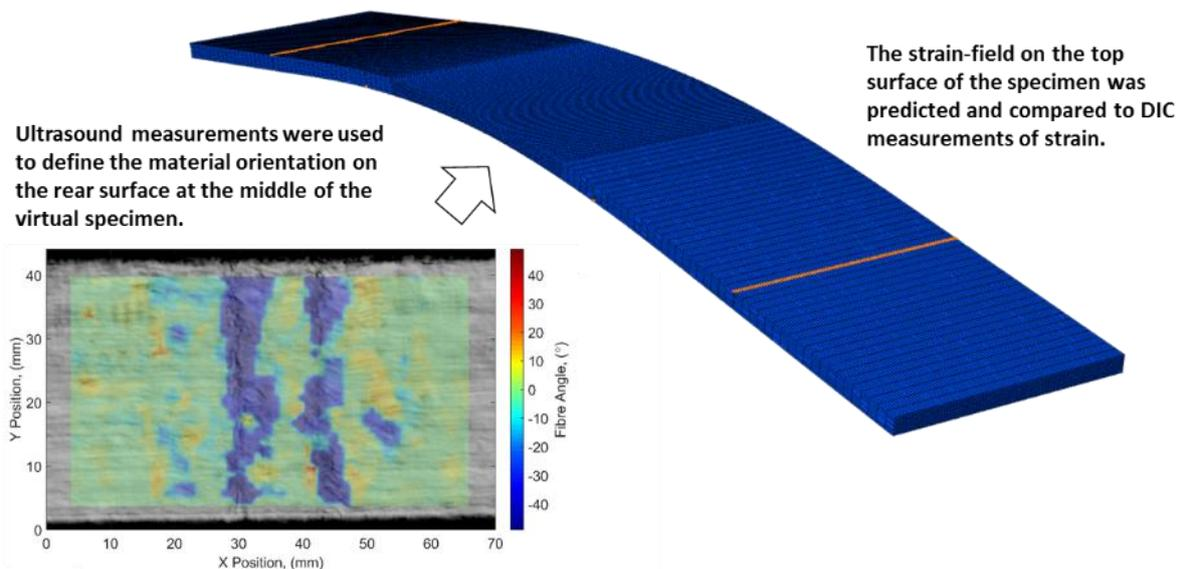
**Fig 1:** Illustration of how fibre orientation measured using ultrasound (bottom left) was incorporated into the model (top right).
