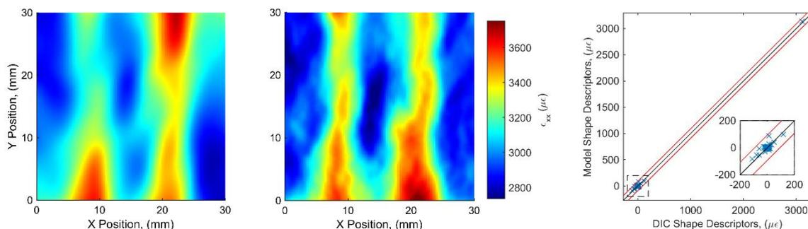
**Fig 2:** Predictions of surface strain (left) and DIC measurements (centre). The validation diagram (right) shows that the model is valid given the uncertainty of the measurement system, the inset shows an enlarged version of the boxed region on the main graph.
