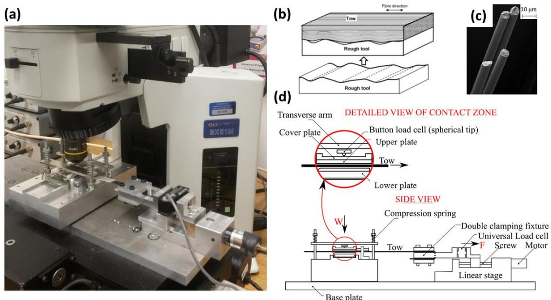
Fig.1: (a) Photo of experimental rig in-situ on microscope stage, (b) schematic of tow-tool contact, (c) SEM micrographs of individual carbon filaments and (d) Schematic side view of experimental rig.
