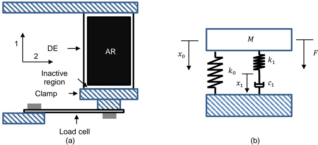
Fig. 1: Schematic diagram for (a) experimental setup and (b) conventional DE model
