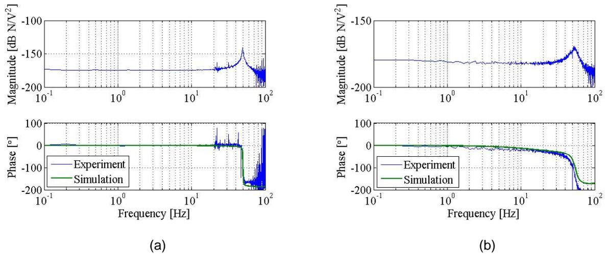
Fig. 2. Bode plot of experimental results in force/voltage<sup>2</sup> over 0.1 Hz to 100 Hz for (a) the silicone-based DEA and (b) the polyacrylate DEA. They are compared with simulation results in phase plot.
